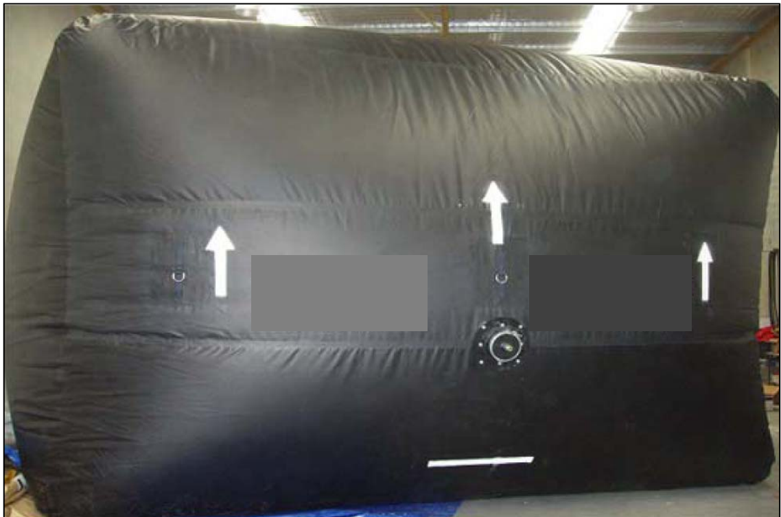
Figure 38: Inflatable roadway seal - Ventstop
