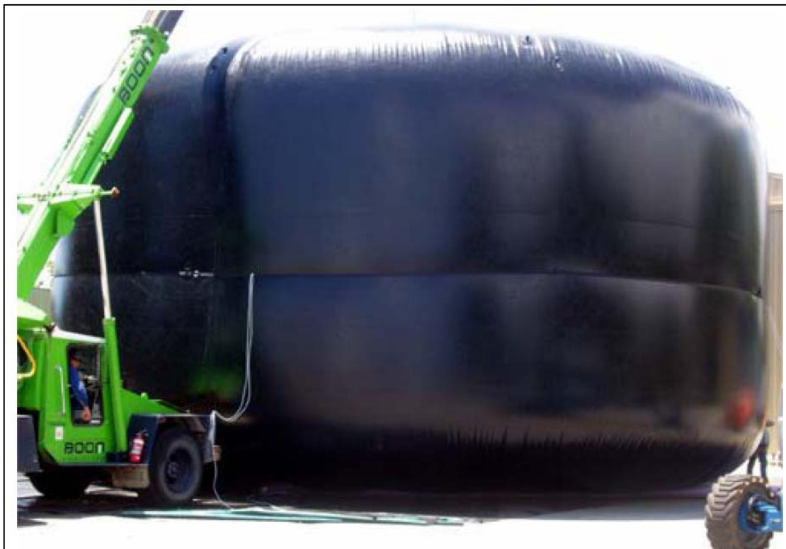
Figure 37: Inflatable Shaft Seal
